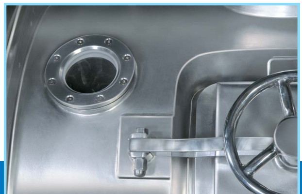
Visual Inspection Port
