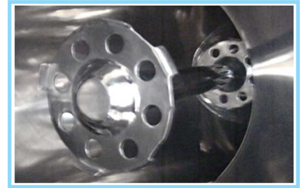
Intensifier Bar with Sprinkle Provision
