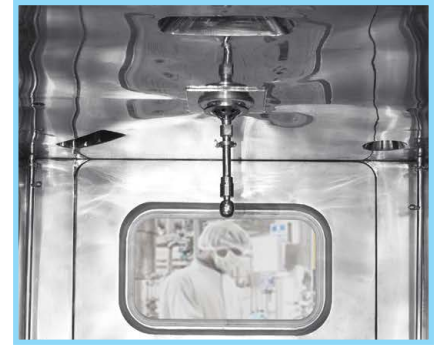
Telescopic Spray Nozzle for Internal Bin Washing
