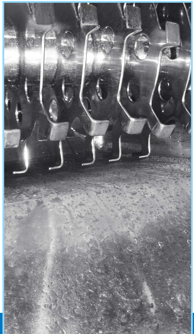
Breaker Blades on Rotating Shaft
