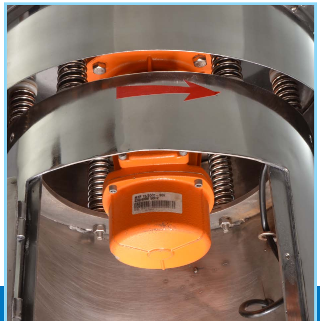
Eccentric Motor for Controlled Vibration
